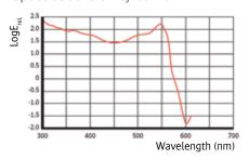
Sensitivity according to the energy necessary to attain a density of 1 above fog
