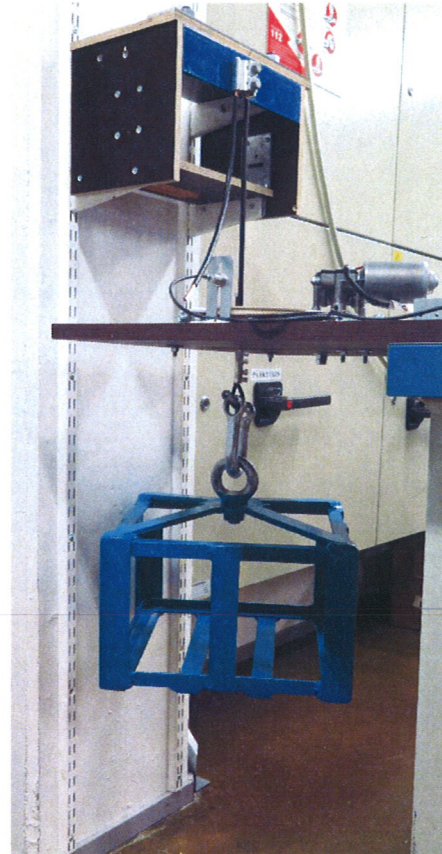
Picture 4: Test setup in pull out test
