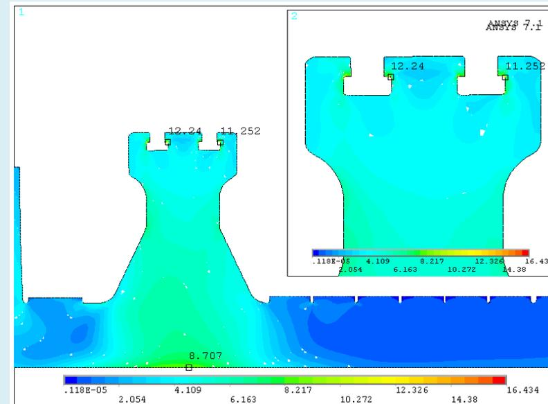
Areas of rotor prone to damage due to creep and low cycle fatigue:
