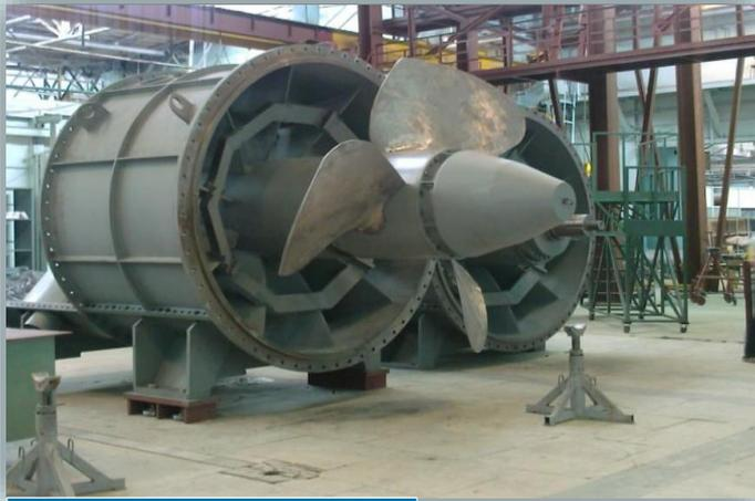
*Variable-speed hydroelectric unit for Mitu HPP (Colombia)*
