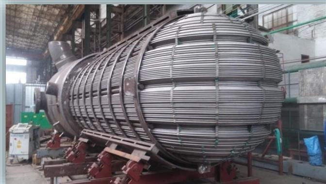
**Absence of water mass in the steam space of the heater is advantage of horizontal design. It decreases a possibility of moisture entering the turbine and turbine rotor overspeed, i. e. overall reliability of the turbine increases.**
