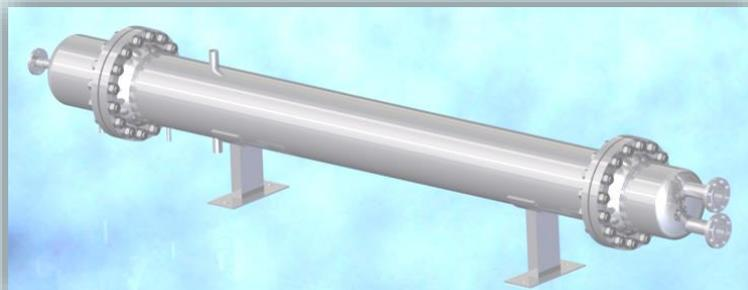
Heaters of PMRN type provide heating of M100 fuel oil to the temperature of **60 to 135 °C**, have capacity of **6 to 400 t/h**, higher thermal efficiency and lower hydraulic resistance in comparison with PMR heaters (production which is terminated), and practically match by mounting dimensions.
