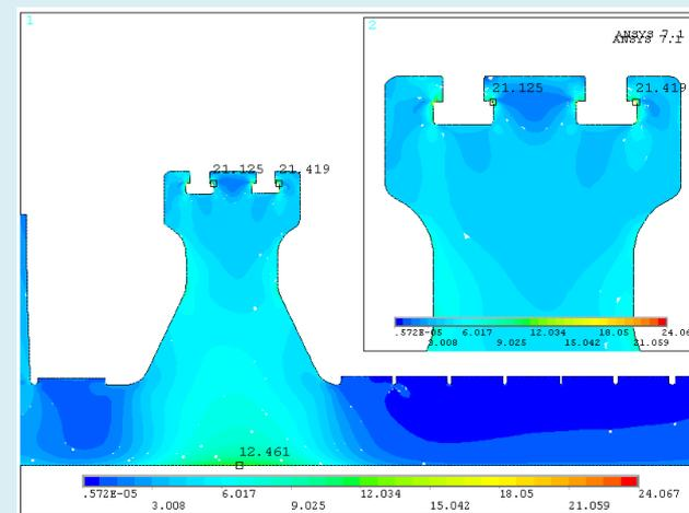
Distribution of equivalent stresses in the rotor section at reference time and with settled creep (kgf/mm<sup>2</sup>)
