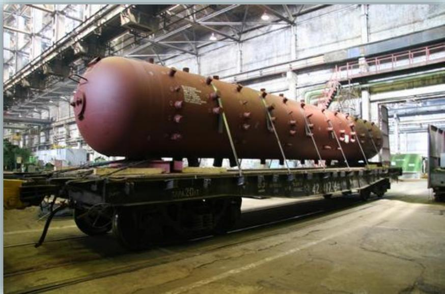
The deaerator design is based mainly on well-known and proven solutions. The use of a jet nozzle as a low-pressure water distributor at the top of the column allows creating an additional contact surface of the water and vapor phases to improve heat and mass transfer and thereby improve performance of the deaerating column. Use of two jet stages in the column and the flooded bubbling device in the tank can guarantee the required water heating and deaeration.
