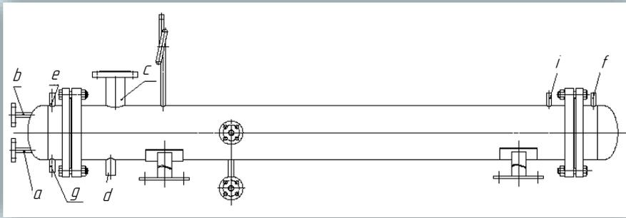
The heaters have capacity of **250–1600 kg/h**, provide heating of M100 fuel oil at nominal flow rate to the temperature of **70 to 95 °C** at the steam pressure of **10 kgf/cm<sup>2</sup>**. The heaters are designed for fuel oil pressure of **25 kgf/cm<sup>2</sup>**. PPM heaters have a built-in cooler of heating steam condensate.
