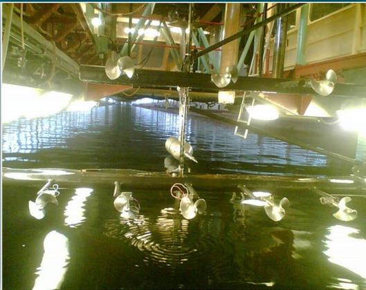
*Frame with hydrometric propellers*
