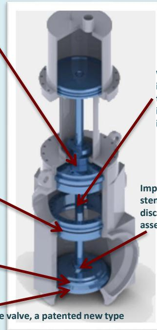
When intake valve is triggered, the stem stability is provided preventing its deflection
