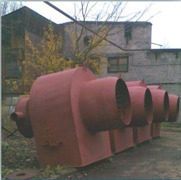
*Oil-gas burner GMU-m with tubular gas distribution*
