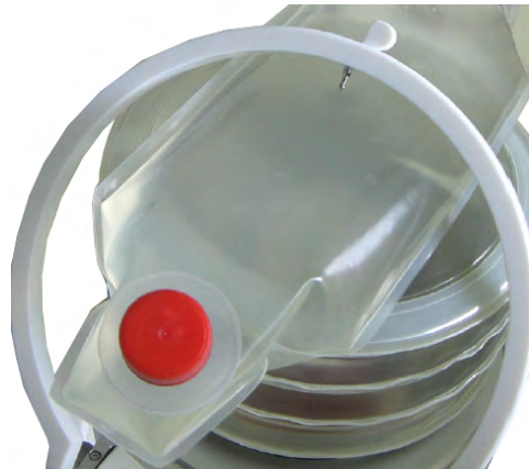
Fig. 12-5 Contact between the reflection mark and focus check water pillow
