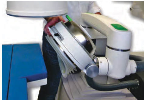
Fig. 5-1 Inspecting the load compensation mechanism
