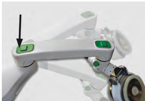
Fig. 8-5 Unlocking the therapy arm
