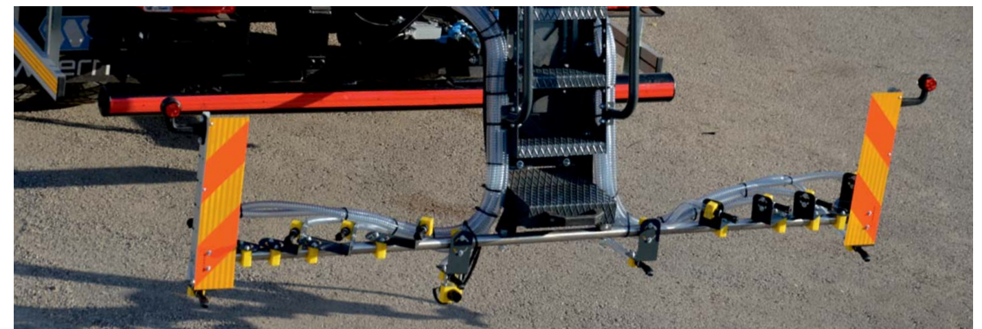
Stainless steel foldable spray bar, 12 liquid spraying nozzles for multi-lane and high speed spraying
