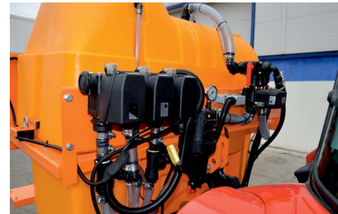
Liquid control valves and installation
