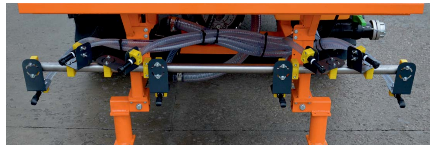
Stainless steel spray bar, equipped with 8 liquid spraying nozzles
