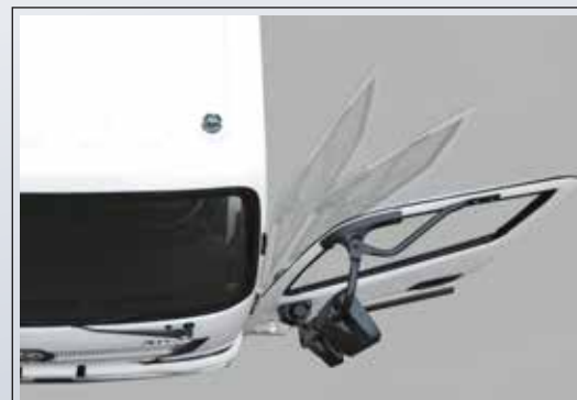
Reinforced doors gradually opening to 90°
