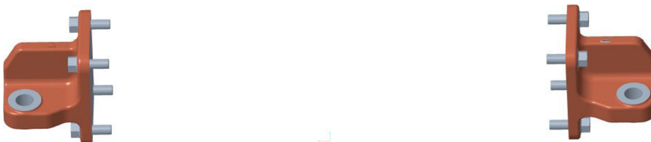
Figure 18: Rear side of pad rear engine support
