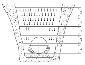
care not to remain empty areas under the pipe and that the lateral parts between the pipe and the walls of the excavation are continuous and compact (layer L1).
