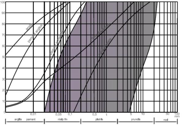
**Horizontal:** The diameters of the granules that correspond to the inner dimensions of the sieve meshes (mm); **Vertical:** Cumulative weights of the fractions that passed through the sieve, calculated as a percentage of the total weight (%)
