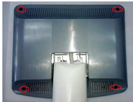
Figure 7-6 Diagram for Dismounting of Rear Cover of Display
