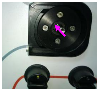
Figure 7-22 Diagram for Dismounting of Pump Assembly(三)
