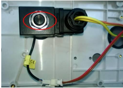
Figure 7-15 Diagram for Dismounting of Valve Assembly
