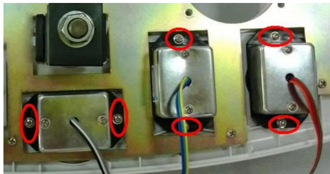
Figure 7-14 Diagram for Dismounting of Air Detector Modules
