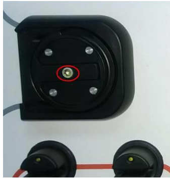
Figure 7-20 Diagram for Dismounting of Pump Assembly(一)
