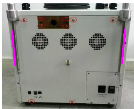
Figure 3-1 Removal of the Host Rear Cabinet
