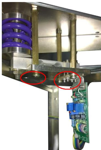
Figure 7-23 Diagram for Dismounting of Electronic scale assembly
