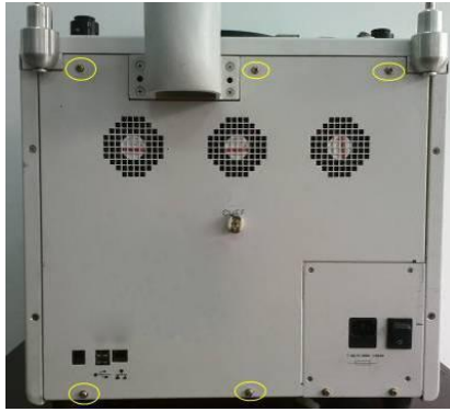
Figure 3-5 Host Rear Cabinet Installation
