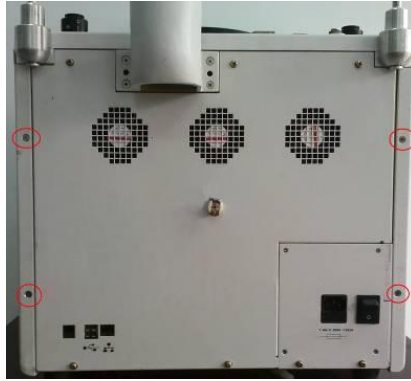
Figure 7-5 Diagram for Dismounting of Left Side Plate and Right Side Plate of the Host
