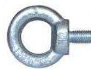
Bulon zincat cu inel: incarcare max. in kg:340 d=12mm
