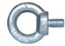
Bulon zincat cu inel: incarcare max. in kg:340 d=12mm
