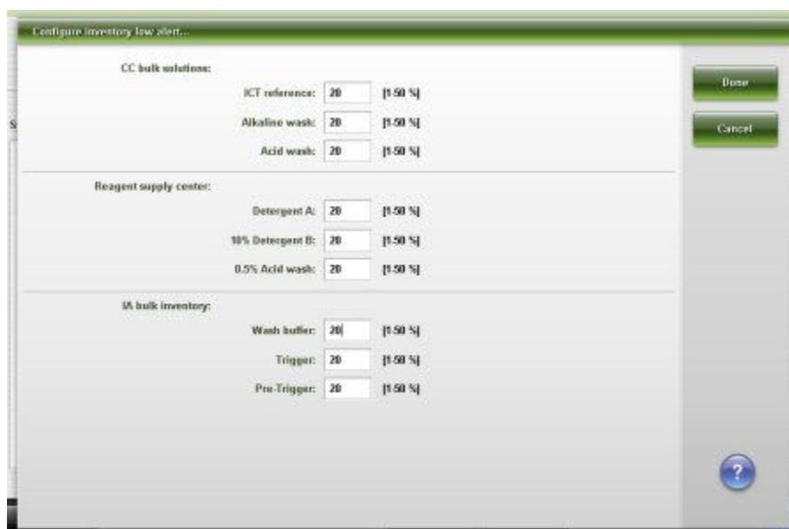
**Figure 2.10: Configure inventory low alert window (c16000/i2000/i2000SR)**
