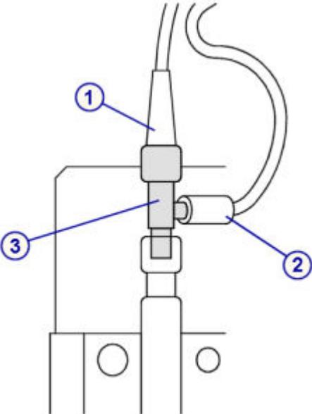
A technical diagram showing a syringe assembly with tubing. The top part of the syringe is labeled with a circled '1'. A side port is labeled with a circled '2'. The check valve assembly is labeled with a circled '3'. The diagram shows the tubing being reattached to the check valve. |
