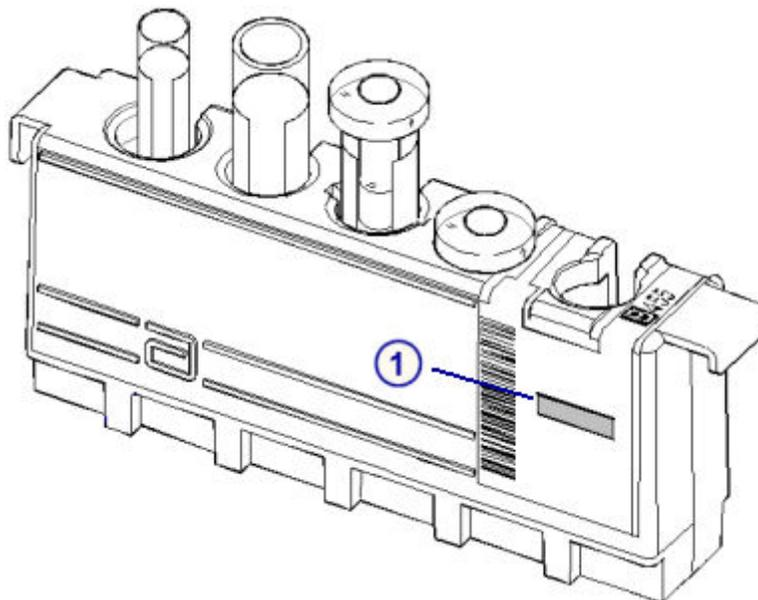
4. Verify adequate sample volume in an aliquot tube by using the sample gauge label (1 on the illustration).
