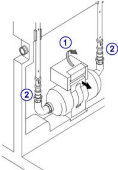
A technical line drawing of a buffer filter assembly mounted on a wall. The assembly consists of a cylindrical filter unit with two grey quick disconnects on either side. A bracket is mounted on top of the filter. A hand is shown pressing down on the bracket, labeled with a circled '1'. Two grey quick disconnects are shown being disconnected from the filter, labeled with circled '2's. Arrows indicate the direction of the hand's force and the disconnection points. |
