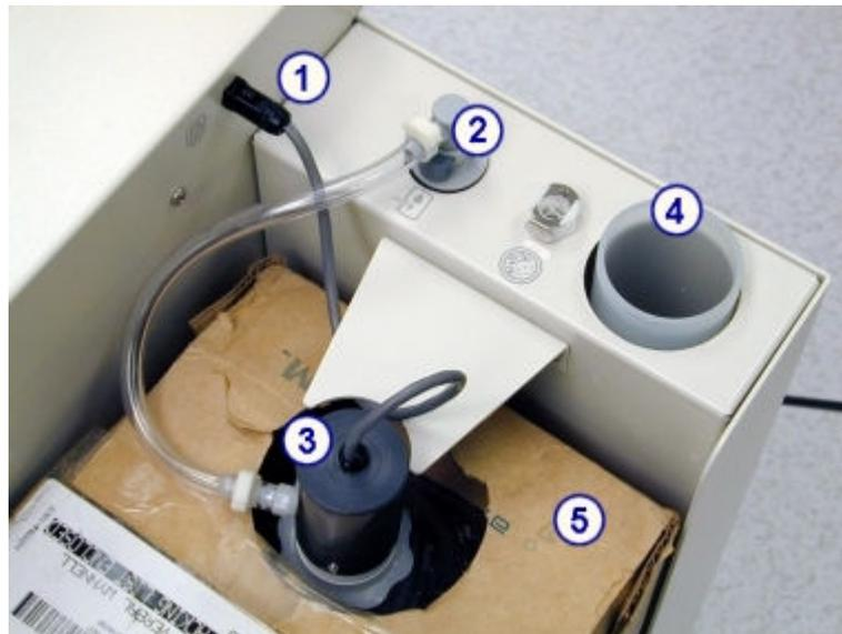
4. Remove the tubing assembly [3] from the concentrated wash buffer cubitainer and place it in the tubing assembly holder. [4]
