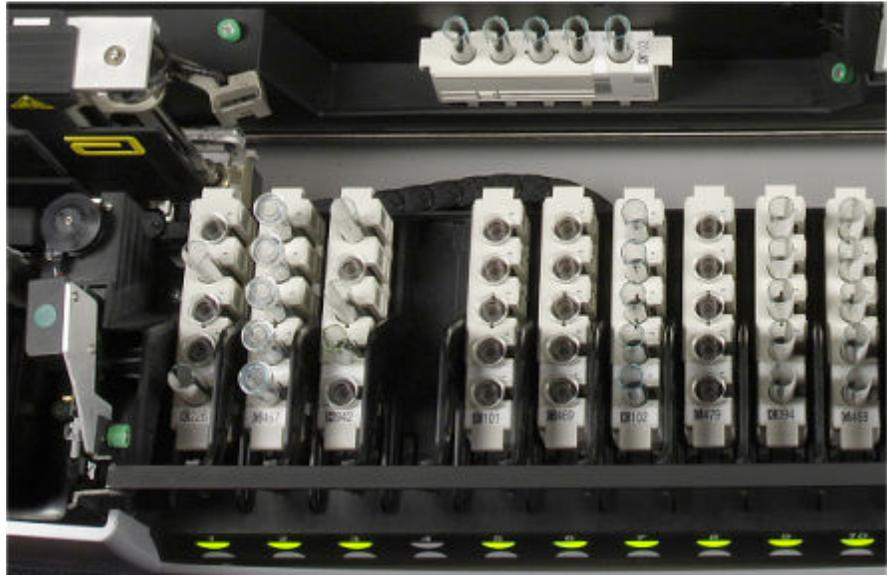
2. Remove the carrier(s) carefully by lifting them up and out of their location.
