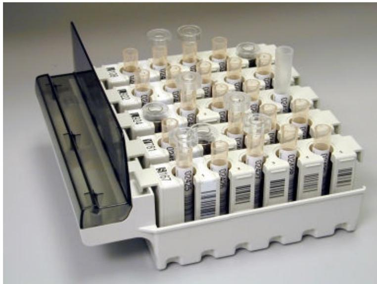
2. Verify the sample carrier(s) sits flush with the bottom of the tray.
