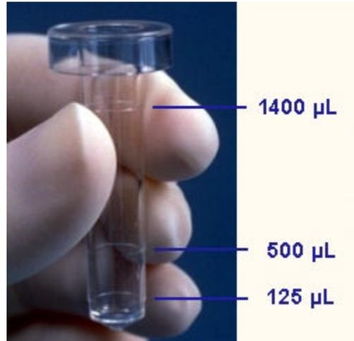
**Figure 5.65: Aliquot and primary sample tube specifications**
