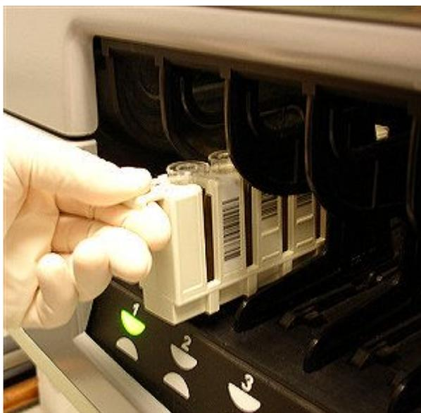
3. Verify the indicators below the routine section farthest to the left are both off, which indicates the section is available.
