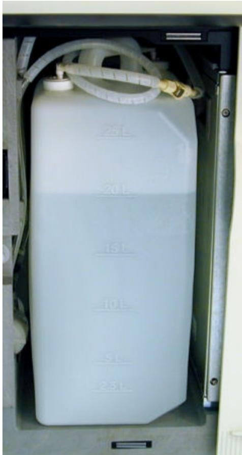
**Wash buffer level sensor and wash buffer inlet assembly (i2000/i2000sR)**
