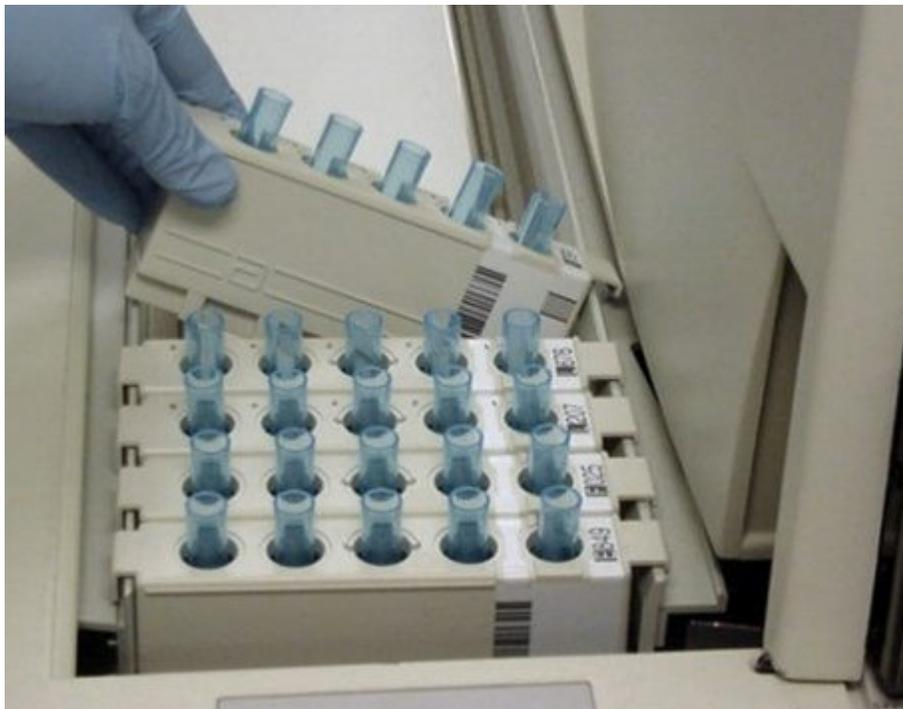
4. Place the sample carrier in the sample load queue by aligning the rail guides over the rails.
