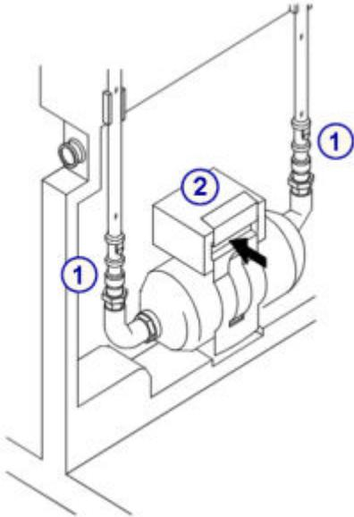
A technical line drawing of a buffer filter assembly mounted on a wall. The assembly consists of a cylindrical filter unit with two grey quick disconnects on either side. A bracket is mounted on top of the filter. A hand is shown connecting the grey quick disconnects to the filter, labeled with a circled '1'. The bracket is shown being pressed into place on top of the filter, labeled with a circled '2'. Arrows indicate the direction of the hand's force and the connection points. |
