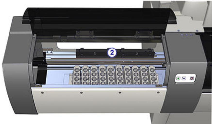
3. Remove or load sample carrier(s) in the area by carefully lifting them up and out of their location or placing them into their location. When loading a sample carrier, place it into position with the sample bar code label window facing the back of the instrument.
