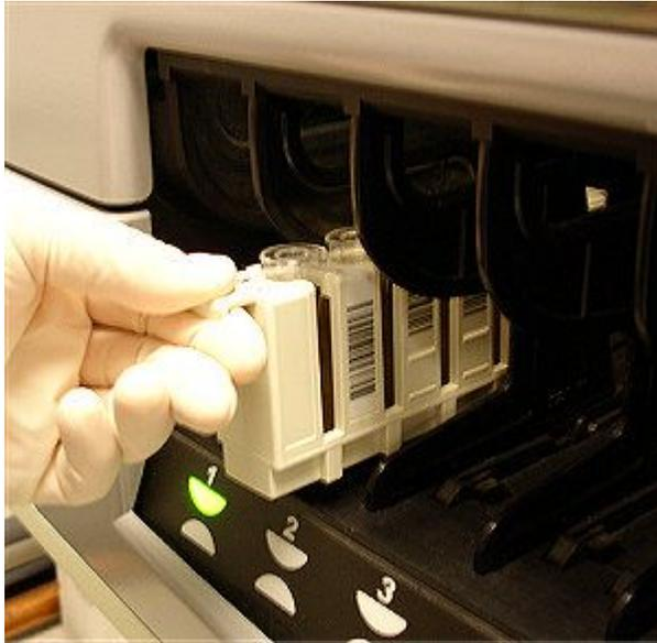
3. Load the carrier into a priority section or a routine section by pushing it in until the indicator illuminates.
