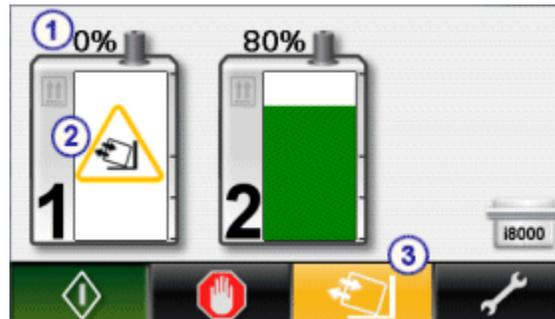
**NOTE:** Do not replace a cubitainer until the Load cubitainer icon displays. The cubitainer is supplying concentrated wash buffer until the icon displays.
