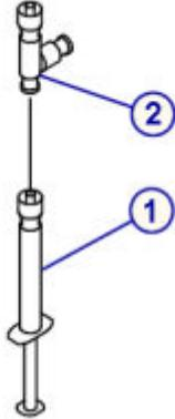
A technical diagram showing two parts of a syringe assembly. The upper part, labeled with a circled '2', is a check valve with a side port. The lower part, labeled with a circled '1', is the syringe body with a plunger. The check valve is positioned above the syringe body, indicating the assembly point. |
