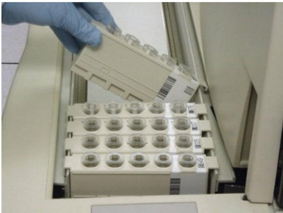
4. Place the sample carrier in the sample load queue by aligning the rail guides over the rails.
