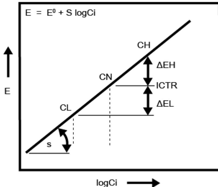
Electromotive force is derived from the Nernst equation,  $E = E^0 + S \log C_i$ , where:
