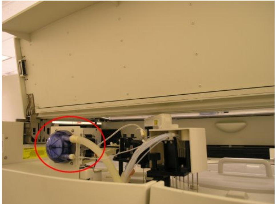
The peristaltic high-concentration waste pump is located in the back under the rear processing module cover.
