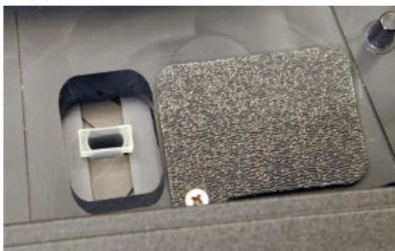
**RV loader and hopper assembly (i2000/i2000sR)**
