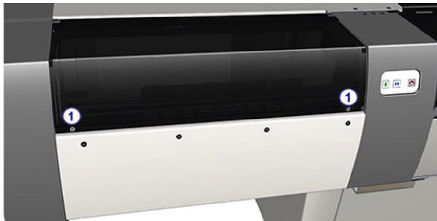
2. Lift the RSHx cover and locate the RSHx carrier exchange area [2].
