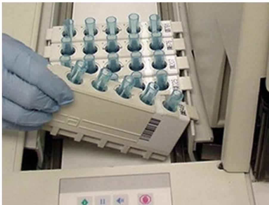
4. Place the sample carrier in front of the carriers currently loaded in the sample load queue by aligning the rail guides over the rails.
