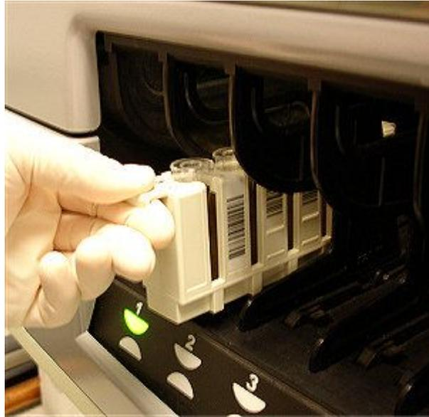
2. Remove the samples from the sample carrier.
