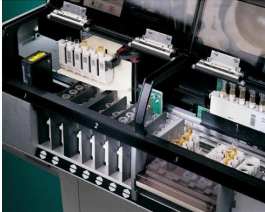
2. Remove the carrier(s) carefully by lifting them up and out of their location.
