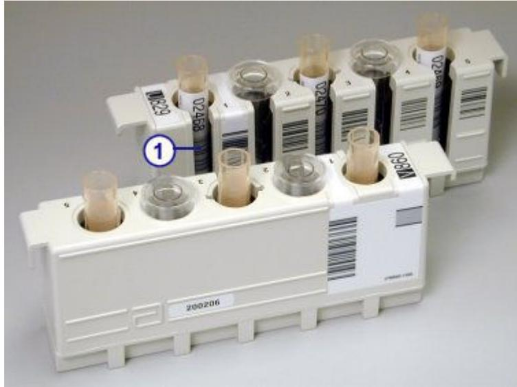
**IMPORTANT:** When you load sample cups and/or tubes, ensure that you have pushed them completely down into the sample carriers and that they are not tilted.
