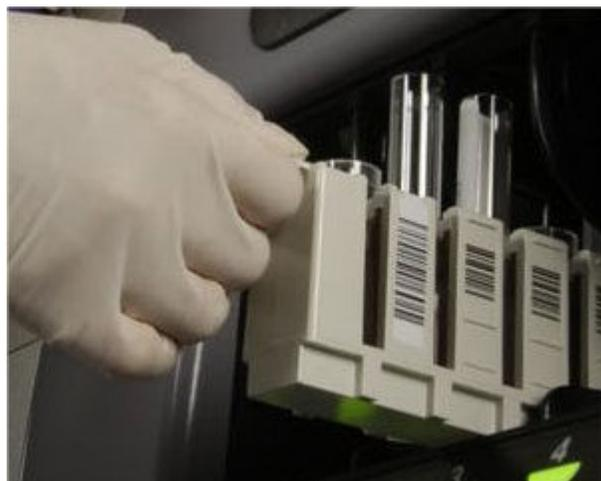
3. Verify the indicators below the routine section farthest to the left are both off, which indicates the section is available.
