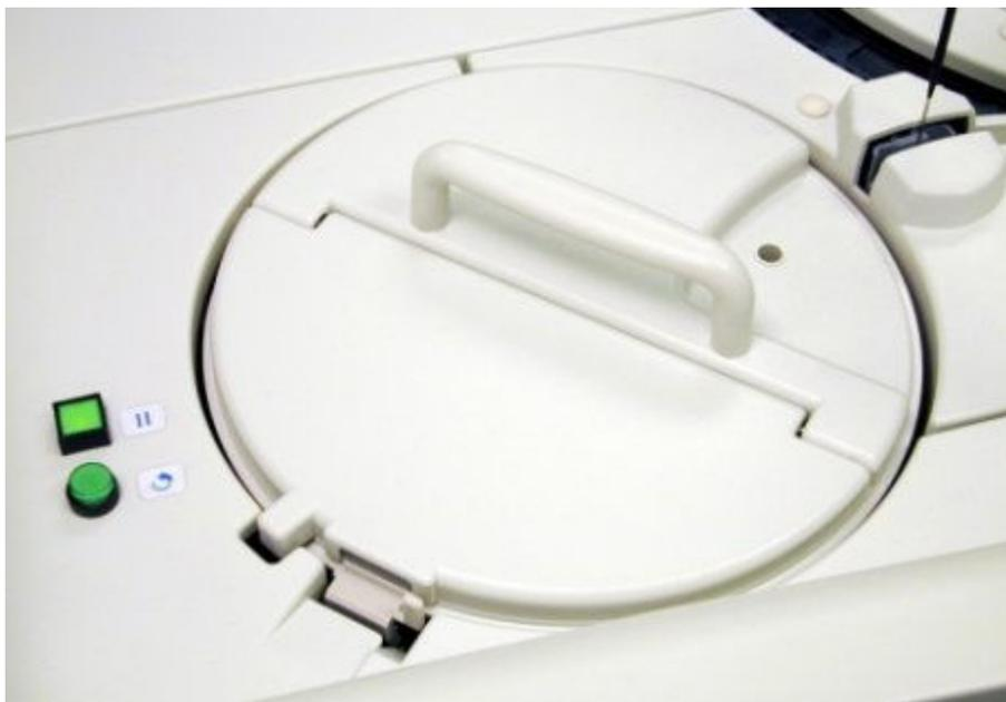
4. Press the **sample carousel advance** indicator button (round) to advance the sample carousel to access the desired position(s).
