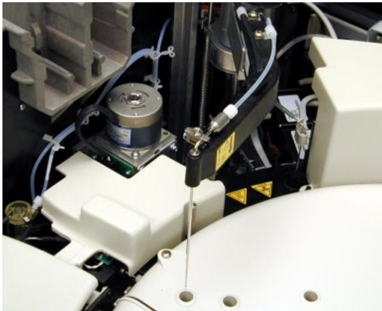
**Figure 1.113: Reagent pipettor (R2 - i2000/i2000sr)**
