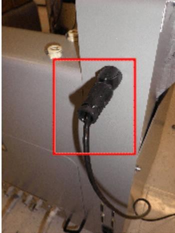
5. Attach the other end of the Filling Station cable to the wash buffer level sensor.
