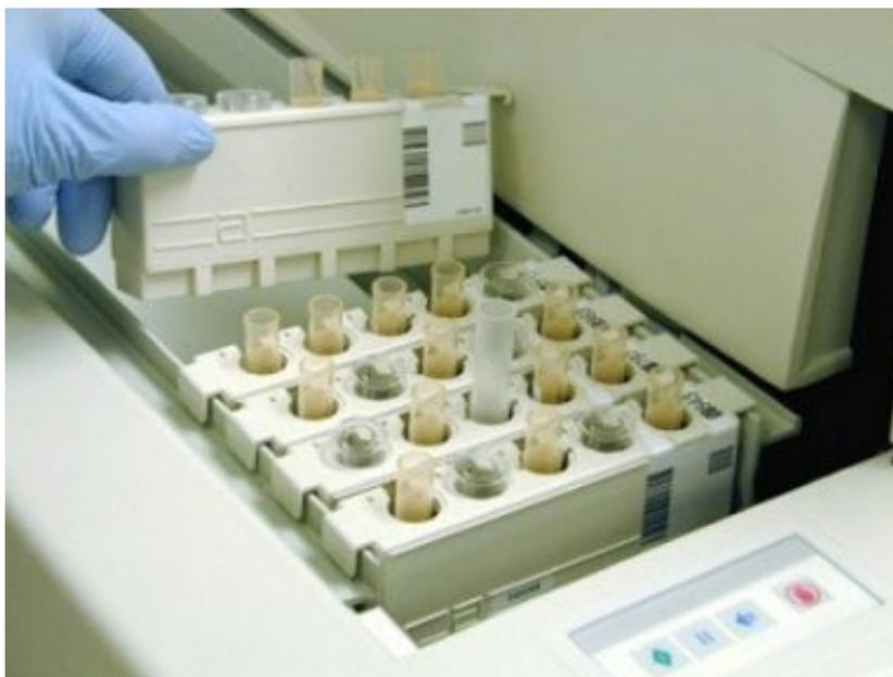
3. Place the sample carrier in the sample load queue by aligning the rail guides over the rails.
