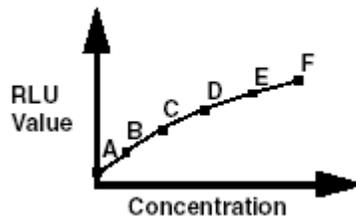
For example, if a sample has an RLU value between the RLU values for Calibrator B and Calibrator C, the unknown sample concentration is calculated using the following equation:
