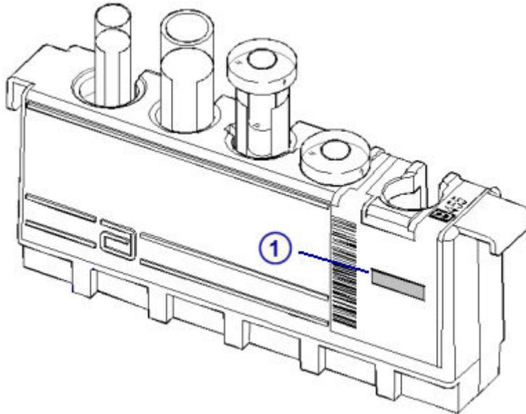
7. Verify adequate sample volume in an aliquot tube by using the sample gauge label (1 on the illustration).
