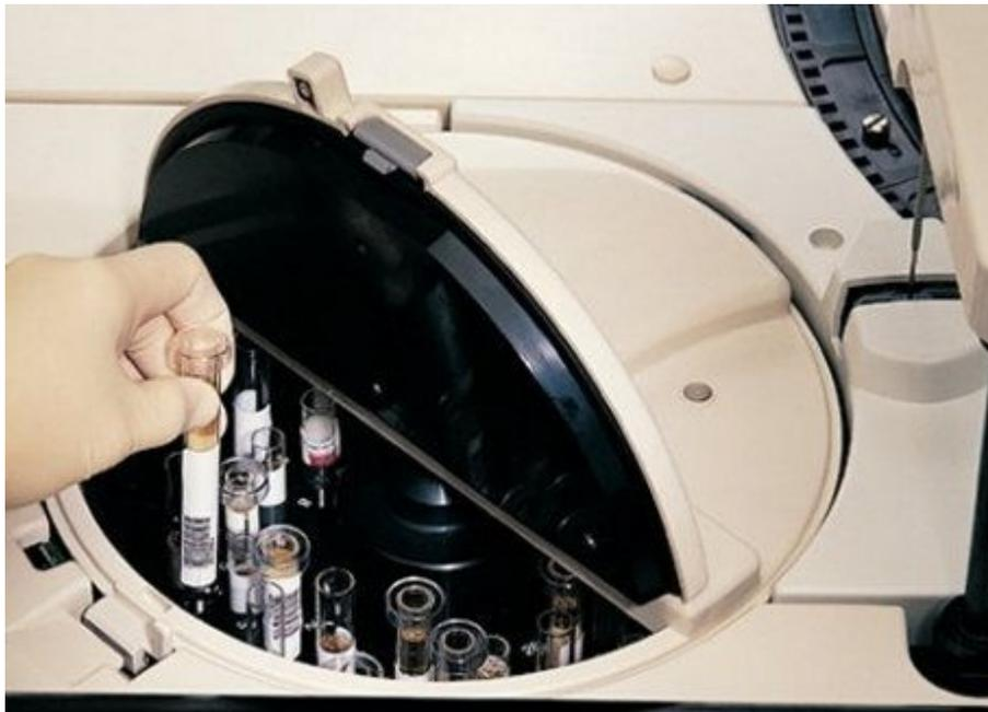
11. Close the sample carousel cover to initiate sample processing by pushing the cover down until you hear a click.
