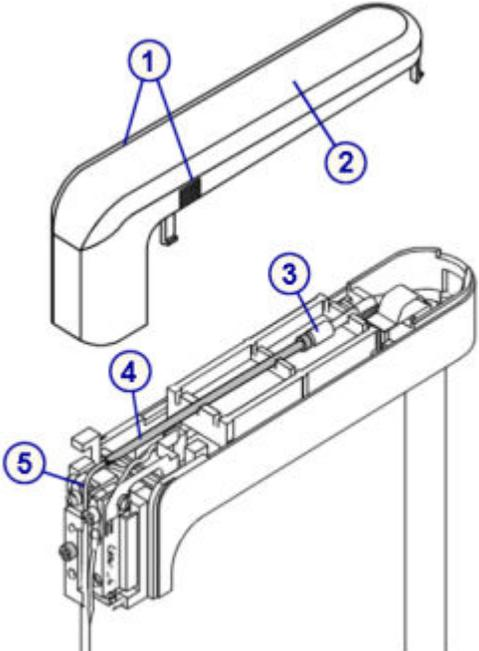
A technical diagram illustrating the removal of sample probe tubing. The diagram is divided into two parts. The upper part shows a sample pipettor cover with two circular callouts labeled '1' pointing to the squeeze points and '2' pointing to a locking tab. The lower part shows the probe assembly with callouts: '3' points to a tubing connector, '4' points to the tubing being disconnected, and '5' points to the top of the probe. |
