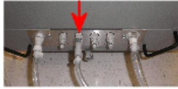
7. Connect the other end of the Filling Station tubing to the wash buffer level sensor.
