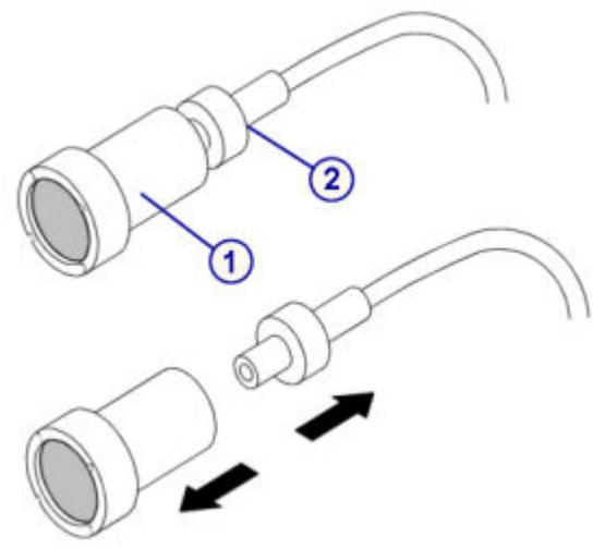
A line drawing illustrating the removal of a filter. A blue circle with the number '1' points to the filter, and a blue circle with the number '2' points to the connector. Two black arrows indicate the direction of movement: one arrow points away from the connector towards the filter, and another arrow points away from the filter towards the waste receptacle. |
