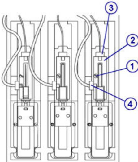
A technical line drawing showing three syringe blocks mounted in a vertical frame. Each block has a syringe plunger and a drive mechanism. Callout 1 points to a slotted screw on the top of the middle block. Callout 2 points to the syringe block housing. Callout 3 points to a knurled connection at the top of the middle block where a tube is attached. Callout 4 points to a knurled connection on the side of the middle block where another tube is attached. |
