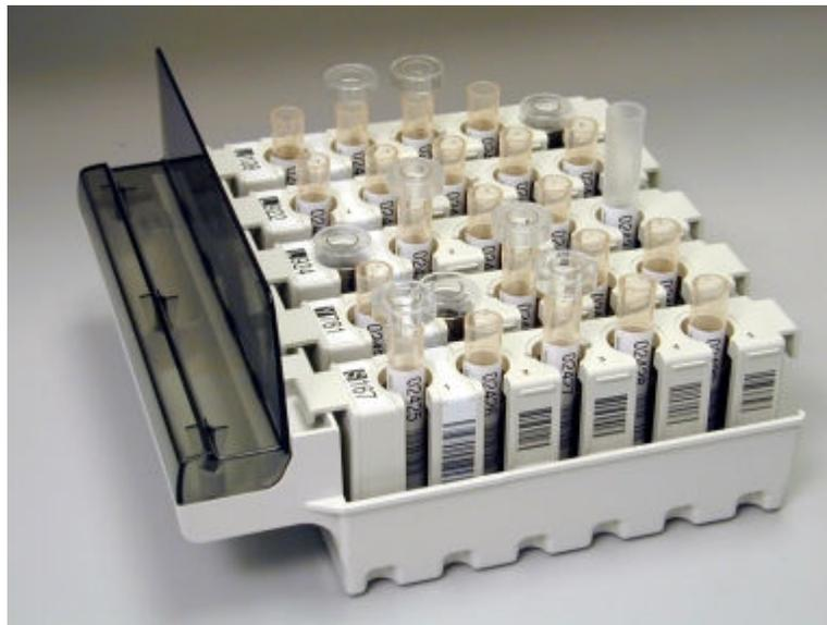
3. Load the carrier into the farthest position on the left side of the tray.
