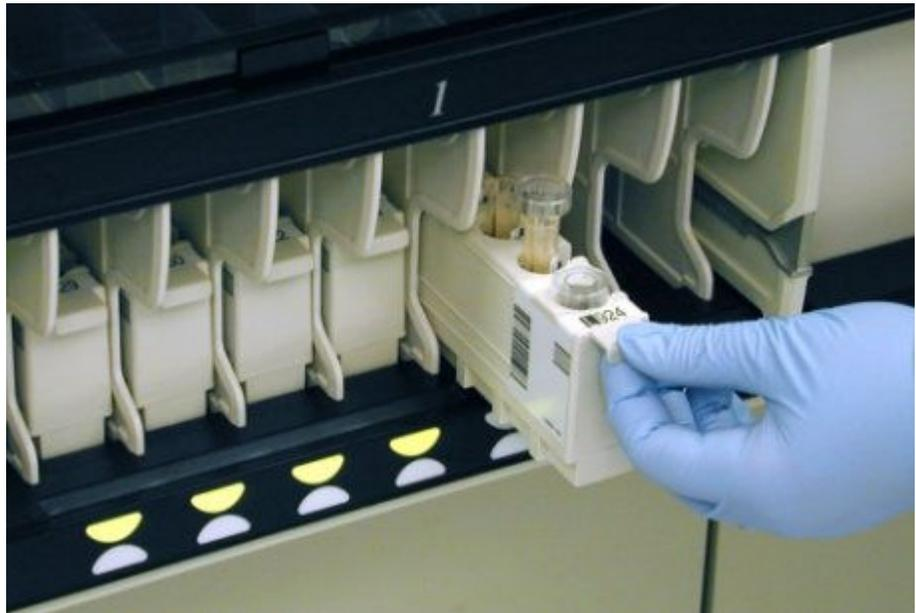
3. Load the carrier into the priority section by pushing it in until the indicator illuminates.
