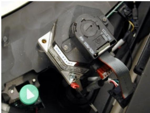
**Pre-trigger/trigger manifold (i2000/i2000sr)**
