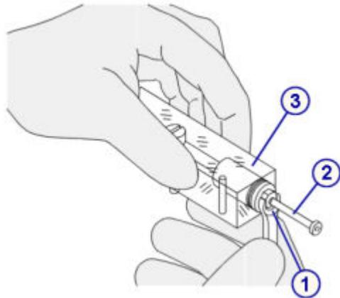
A line drawing showing a hand holding a syringe block. The hand is using a 10 mm wrench to turn a nut (callout 1) located at the bottom of the syringe plunger (callout 2). The syringe block (callout 3) is held steady by the other hand. |
