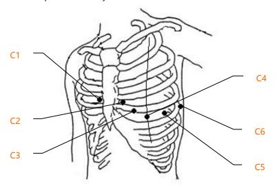
Fig. 4-5 Chest Electrode Positioning
