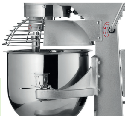
Stainless steel protective guard over the bowl
