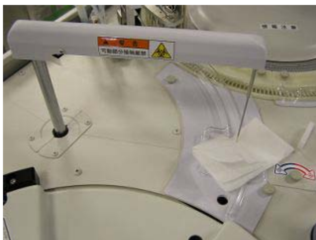
Covering the SPP wash port with 4-5 sheets of Kimwipe
