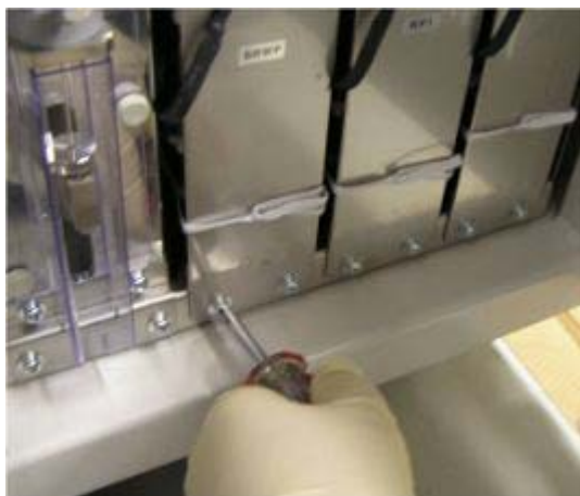
Removing the fixing screws of the pump
