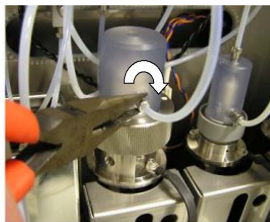
Attaching the joint on the front side of the cylinder
