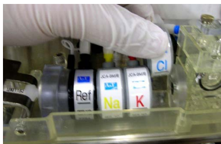
Removing the electrode
