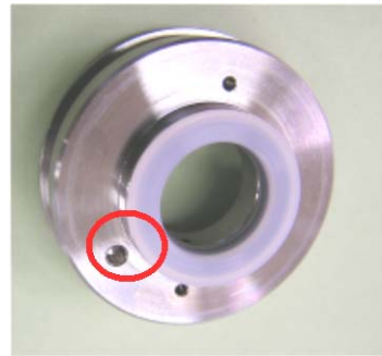
Fitting hole on the spacer
