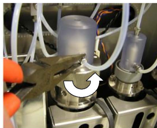
Removing the joint on the front side of the cylinder
