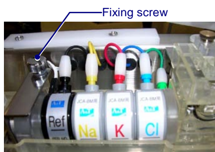
Removing the fixing screw
