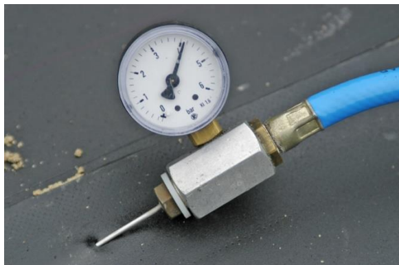
Testing of double seam
