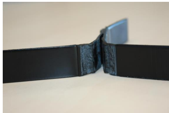
Failed peel test
