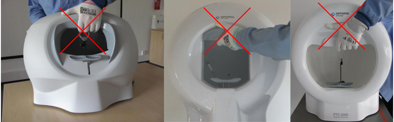
Figure 3. Incorrect way of holding and carrying the perimeter
