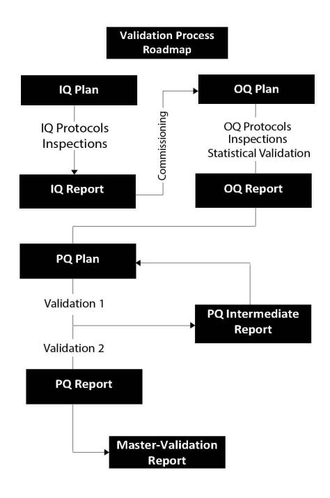
**Performance Qualification:** will commence after satisfactory completion of operational qualification. Optimal setting for autoclave machine will be used and samples will be subjected to clean and results will be determined. When process stability is demonstrated and process gives results in the required range the process will be validated and will be used to control the process.
