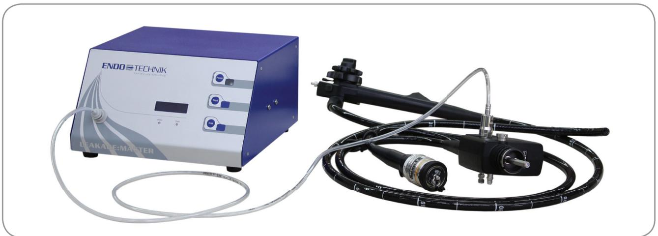
LEAKAGE:MASTER with connected endoscope
