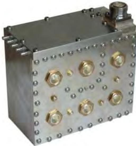
In the MTS 4, the Preselector has an integrated high performance LNA and RMC. The supply voltage for the LNA is supplied through the RX out connected to the Base Radios. The Preselector has outputs for four Base Radios. The antenna connector is DIN 7-16. The receive side is connected by QMA connectors.
