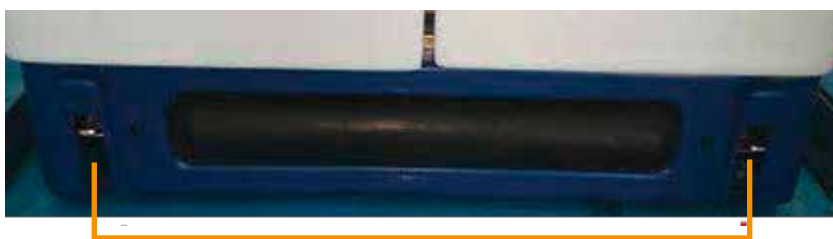
Lever up = unlocked wheels
