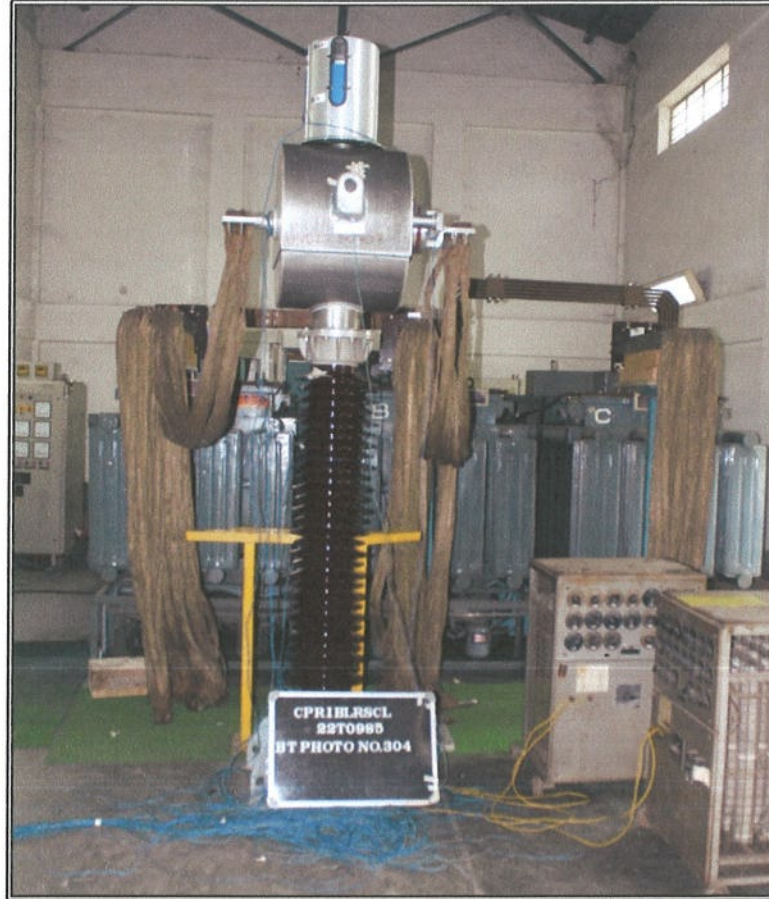
Test arrangement for Temperature Rise test
