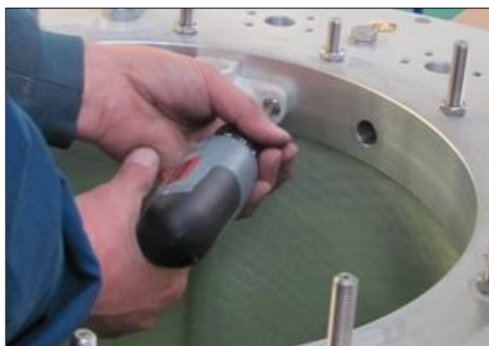
Fig.22 – Uninstalling the siphon of the oil compartment
