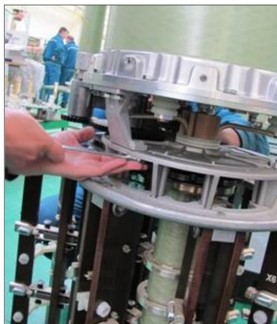
Fig.16 – Connecting the legs of the oil compartment with the selector
