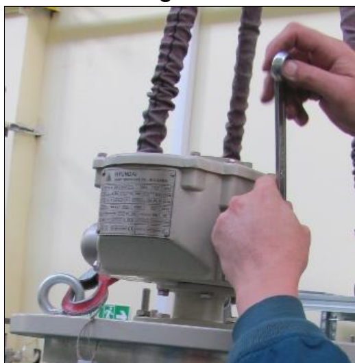
Fig.24 – Turning the incoming shaft of the worm gear box for 8 revolutions
