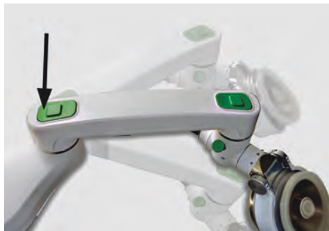
Fig. 8-5 Unlocking the therapy arm
