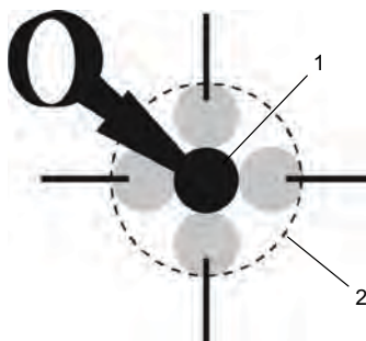
Fig. 11-12 Tolerance range in the Z direction
