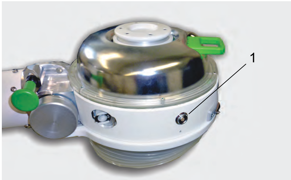
Fig. 3-19 Connector for the in-line unit
