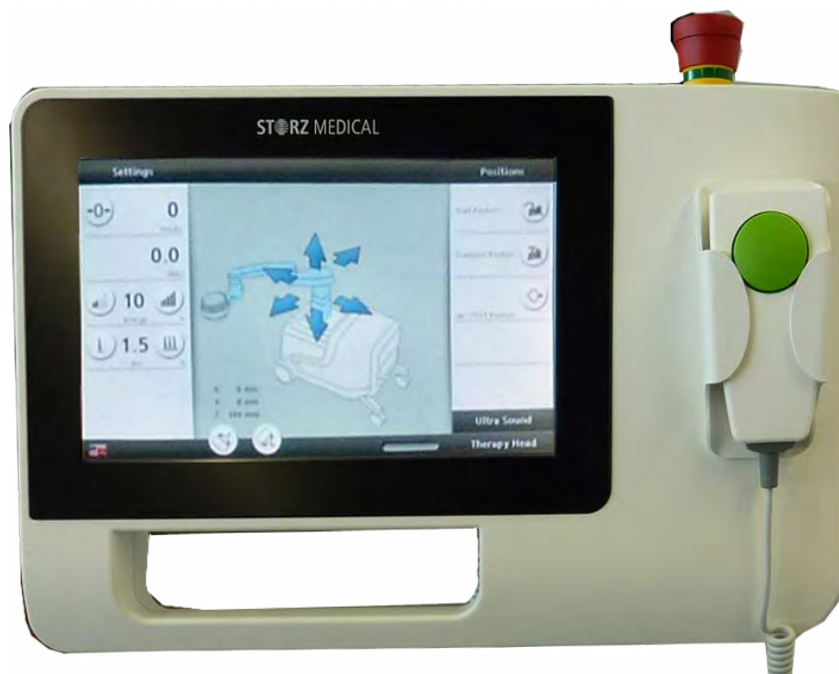
Fig. 3-6 Touchscreen with arrow buttons for moving the therapy arm
