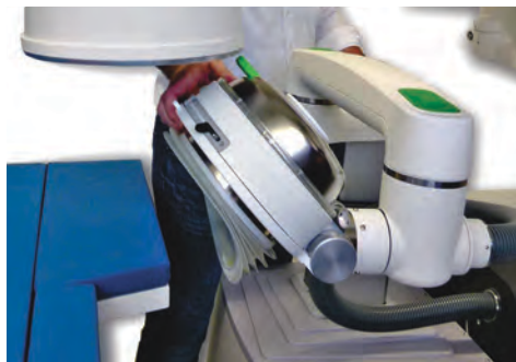
Fig. 5-1 Inspecting the load compensation mechanism
