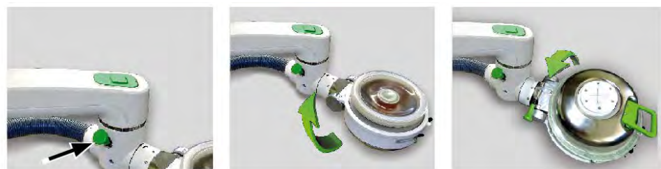
Fig. 3-4 Unlocking the therapy head and rotating it manually
