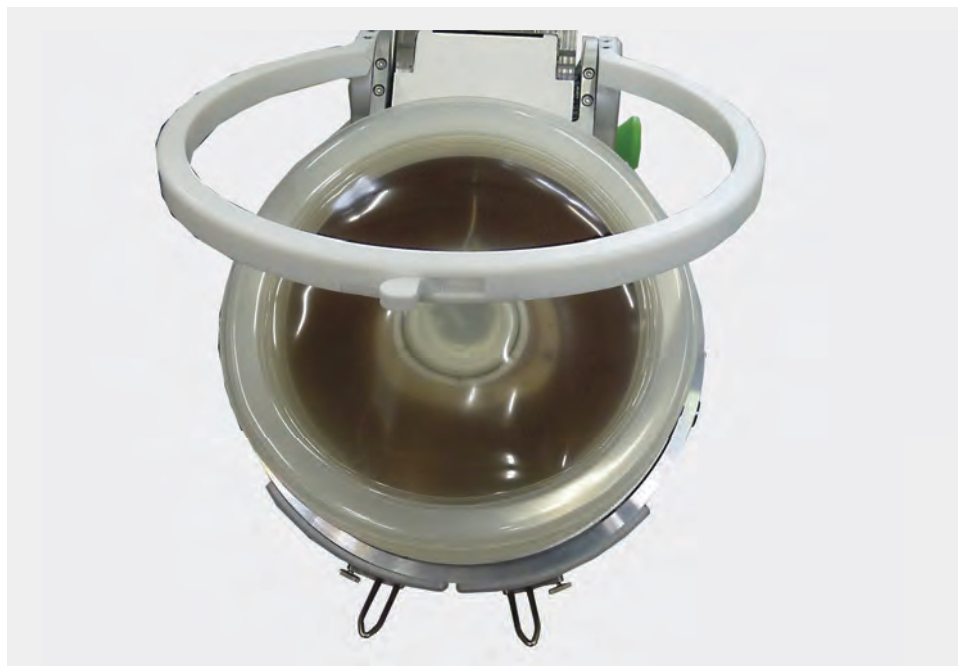
Fig. 12-4 Flipping open the focus gauge
