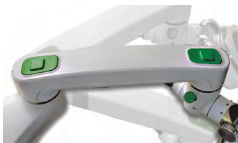
Fig. 11-19 Unlock button on the first joint
