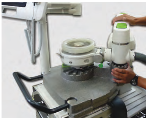
Fig. 8-6 The therapy unit has been placed in the transport position
