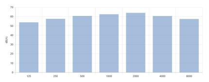
The sound levels are given at full load, without pumps (if available) and at nominal conditions (air temperature: 35,0 °C, water temperature (in/out): 12,0/7,0 °C). Sound power: calculated on the basis of measurements carried out in accordance with the UNI EN ISO 9614-2 regulation, in compliance with the requirements of the Eurovent certification. Sound pressure calculated according to correlation in accordance with UNI EN ISO 3744.
