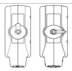
Fig.3-2 a Probe connector "Unlock" status
