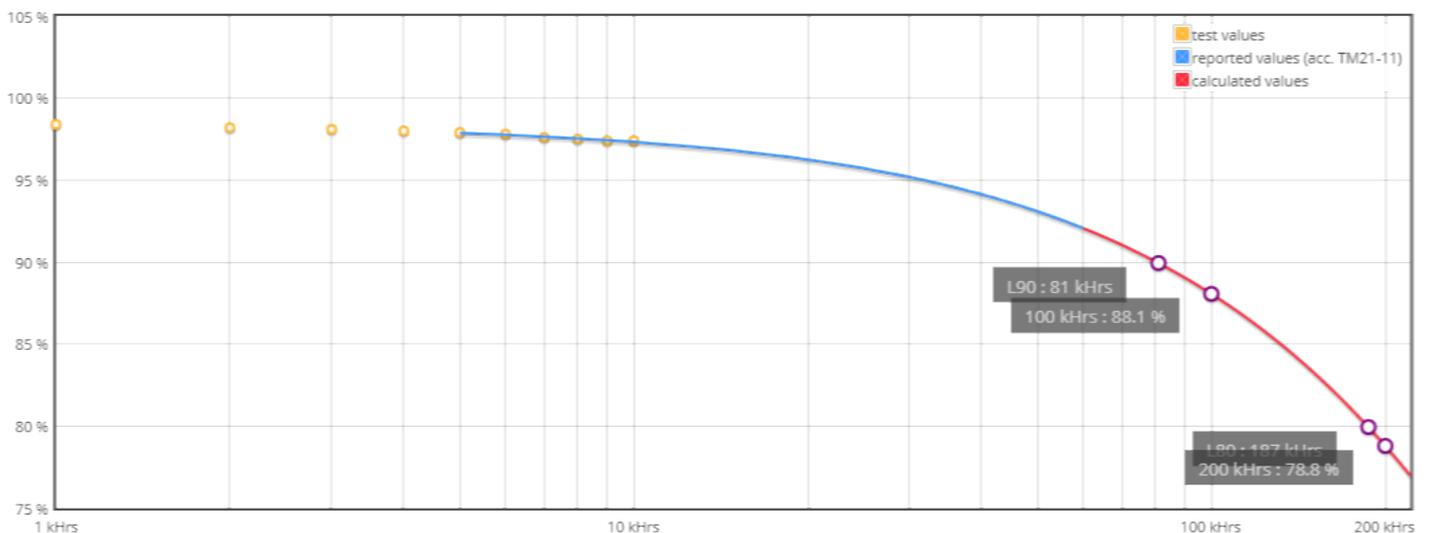
LxB50 results according to LM-80 and TM-21-11 procedures and norms.
