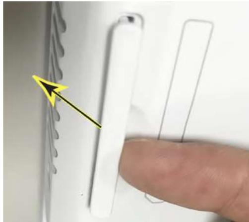
Figure 18-3. Remove the Air Filter
