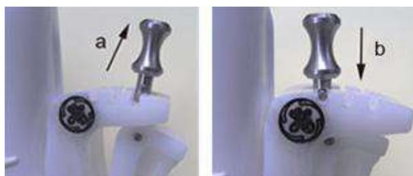
Figure 17-21. Pull up and push down the knob
