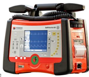
**ILLUMINATED MONITOR** to display 2 ECG curves, vital signs, alarm limits, duration of use, energy levels, mode, pacer, shocks
