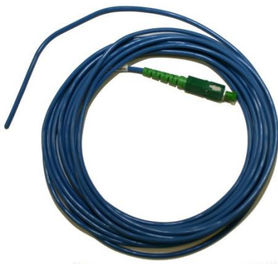
Temperature sensor for intracorporeal (rectum) temperature measurement
