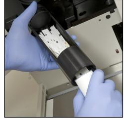
Figure 5: Emptying the unused strip bin back into a test strip vial
