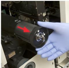
Figure 20: Removing the strip loader cylinder
