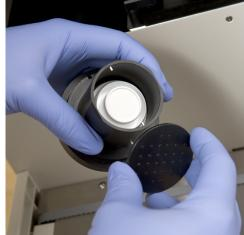
Figure 22: Loading test strips and desiccant into the strip loading cylinder
