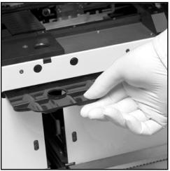
Figure 24: Removing (clockwise) the pipetting stage, the measuring stage, the used strip bin, the drip tray, and the strip comb for cleaning
