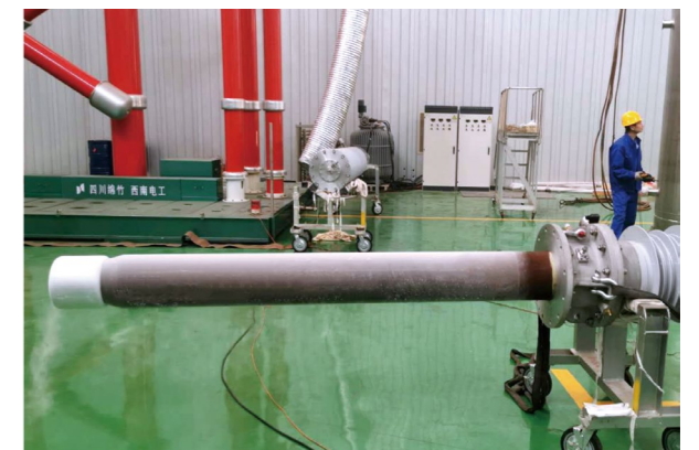
-196°C ~ 室温环境 12 次冷热冲击试验 12 cold and hot shock tests from -196 °C to room temperature
