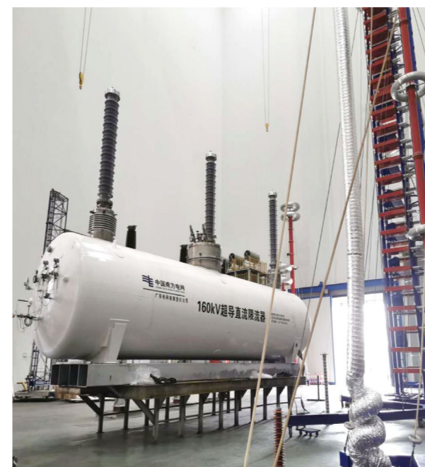
±160kV 直流套管随超导直流限流器试验 Routine test of ± 160kV DC bushing with Resistive-type Superconducting Fault Current Limiter
