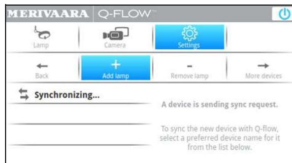
Picture 33. Menu in the main lamp- a device is sending a synchronizing request
