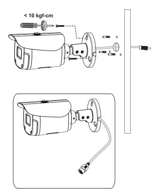
**Note**: It is always a good practice to form a drip loop on cables. Moisture condensation or dripping water can eventually cause problems without the drip loop.
