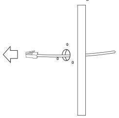
5. Pass an Ethernet cable through the waterproof cable gland components, and through the rubber seal as shown below. Connect the Ethernet cable to the camera's RJ45 connector.
