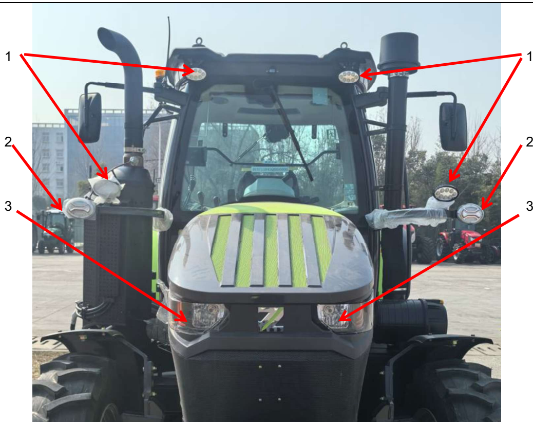
lights installation—front view
