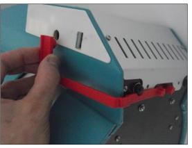
Squeeze the arrows towards each other and while squeezing, pull out the securing device:
