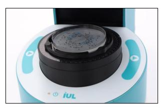
After pushing the button, the diffusing sphere (2) will descend to cover the Petri dish, the lighting and image acquisition procedures will be performed, and finally, the diffusing sphere will return to its upper resting position. Then the process results will be displayed on the screen.
