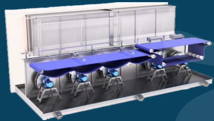
Tunnel Shocking (Blast Freezing)
