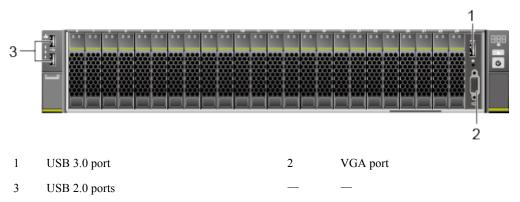
• Figure 4-10 shows the ports on the front panel of a server with 25 hard disks.
