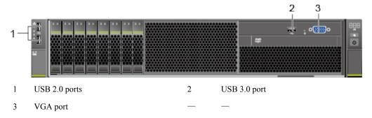
• Figure 4-8 shows the ports on the front panel of a server with 12 hard disks.
