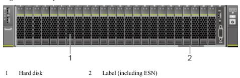
Figure 4-4 shows the front panel of a server with 25 hard disks.
