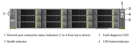
• Figure 4-14 shows the indicators and buttons on the front panel of a server with 24 hard disks.
