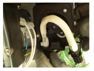
ATTENTION: the rotor of dispensing pump turns ONLY clockwise !!!
