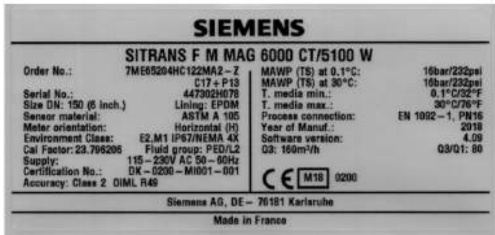
Figure 2-2 Nameplate MAG 6000, 5100 W
