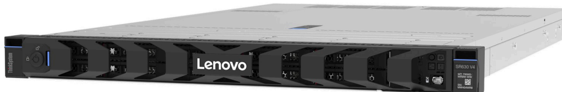
Figure 27. Lockable front security bezel
