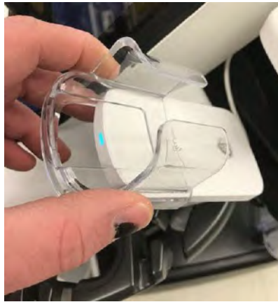
Figure 13-200. Remove Vscan Air Probe Holder
