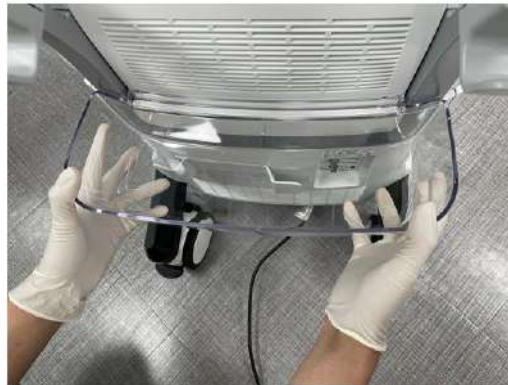
Figure 12-15. Disassemble the rear basket
