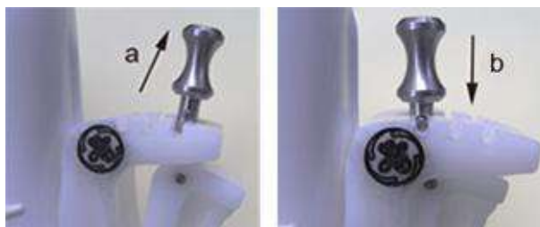
Figure 11-33. Pull up and push down the pin
