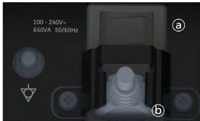
Figure 3-8. Circuit Breaker (a) and Power Plug (b)
