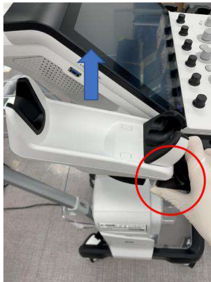
Figure 12-16. Pull the hook to disassemble the probe holder
