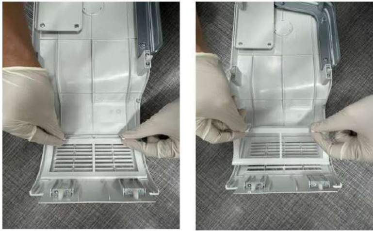
Figure 12-12. Remove the air filter
