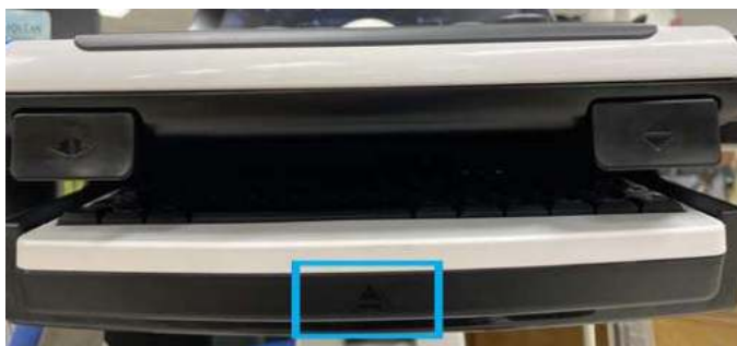
Figure 3-33. Push the keyboard
