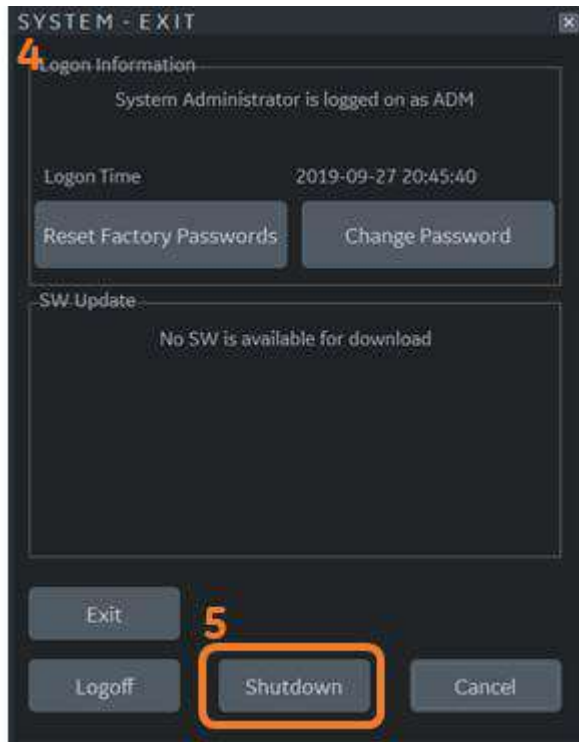
Figure 13-278. Shutdown to Begin Installation
