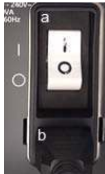
Figure 3-9. Circuit Breaker (a) and Power Plug (b)
