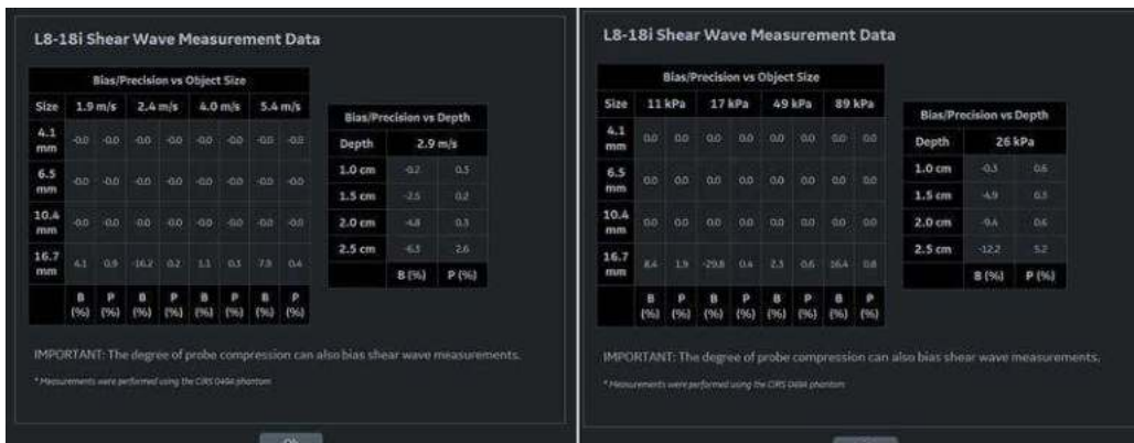
Figure 13-66. L8-18-D Measurement Bias Information (Velocity on the left and Stiffness on the right)
