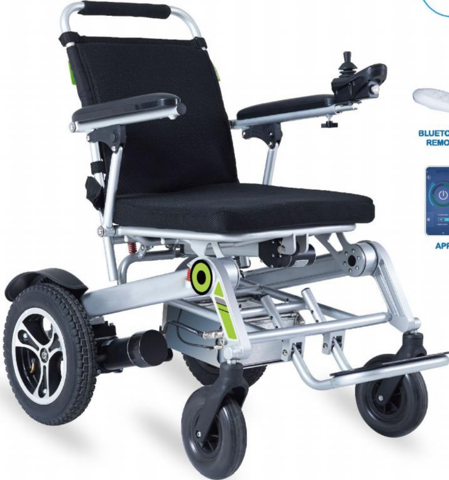
JL-H3 FULLY AUTOMATIC INTELLIGENT FOLLOW WHEELCHAIR, INTELLIGENT JOYSTICK CONTROLLER,EASY AND COMFORTABLE STEERING EXPERIENCE,INTELLIGENT BRAKE,CONTEOLLER CAN BE MOUNTED ON LEFT OR RIGHT ARMREST,ARMREST CAN BE RAISED FOR EASY SIDE ACCESS TO THE SEAT, FOOTREST ADJUSTABLE WITH 3 DFFERENT HEIGHT,DC BRUSH MOTOR,PRESS THE HORN TO GIVE OTHERS REMINDER.
