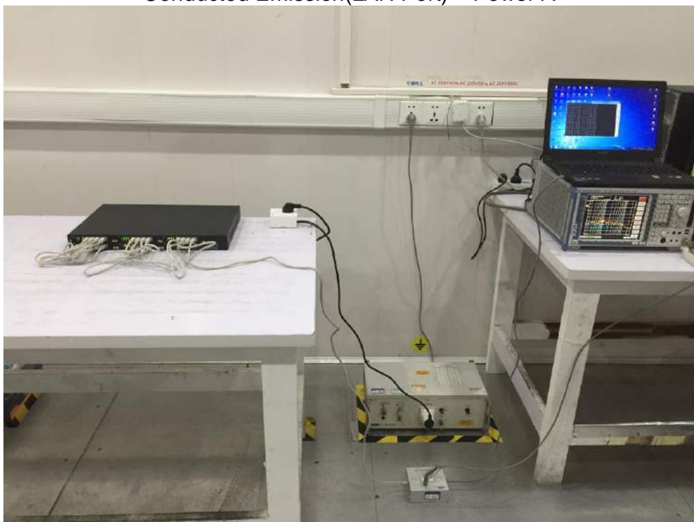
Conducted Emission(LAN Port) – Power A
