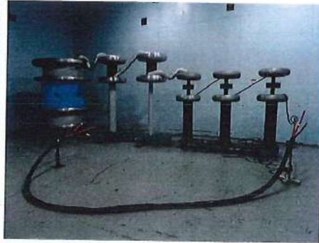
E2: 样品局部放电试验及交流耐压试验 Partial discharge test and AC voltage test on the sample
