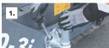
Fit the two brackets to the screed arm.
