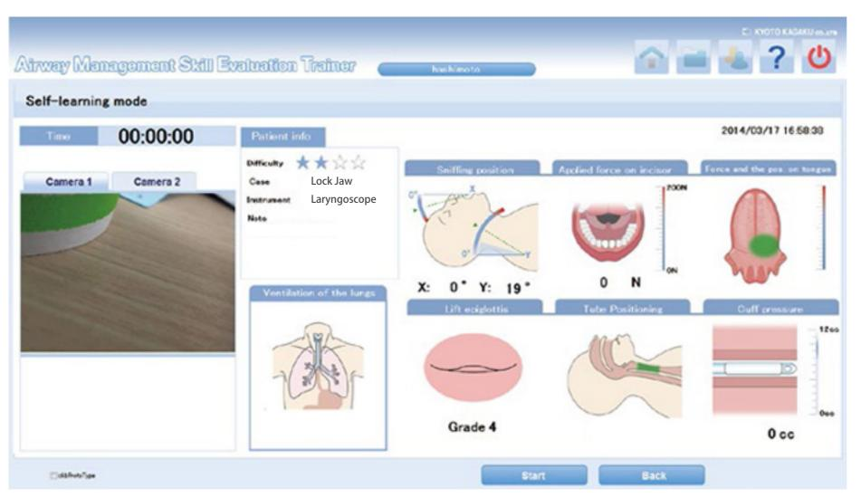
Adjust the camera to capture your hand motions for assessment recording as the image is displayed.
