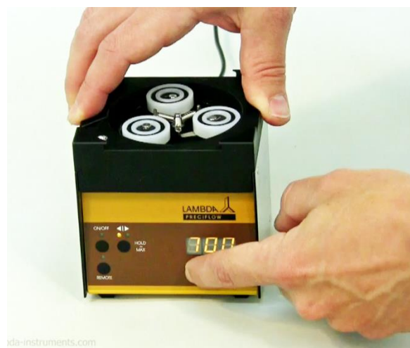
Figure 1-4 The speed of rotation has to be increased using the “^ ^ ^” arrows present below the LED display. Set the pump speed to about 700. The speed range of about 300-700 for tubing insertion can be used.
