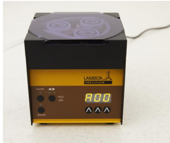
Figure 3-4 The message “A” and two numbers will appear on the display. This number from 00 to 99 is the current address of the pump.
