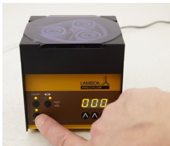
Figure 3-2 Press the button REMOTE on the front panel. The corresponding LED diode will go on and the display will indicate the approximate voltage of the external signal.
