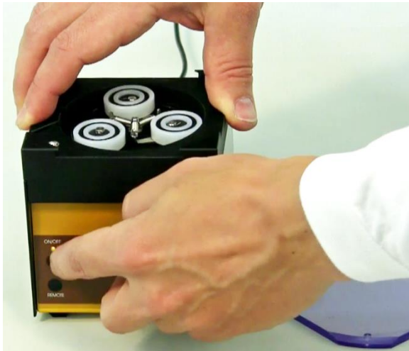
Figure 1-5 Press the ON/OFF button and select the sense of rotation of the peristaltic pump by pressing the button ◀▶
