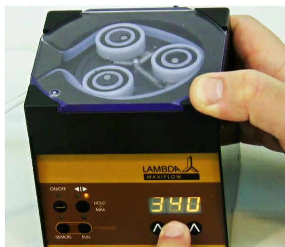
Figure 1-12 Each ▲▲▲ arrow can be used to change the corresponding digit on the flow rate.
