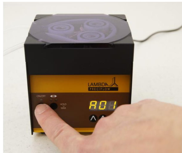
Figure 3-6 To confirm the address and save it, press the ON/OFF button.
