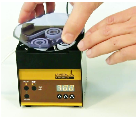
Figure 1-9 Replace the transparent cover by placing it back on the top of the peristaltic pump.
