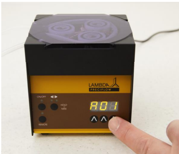
Figure 3-5 To change the address press the buttons ▲ ▲ ▲ under the display until the desired number is obtained.
