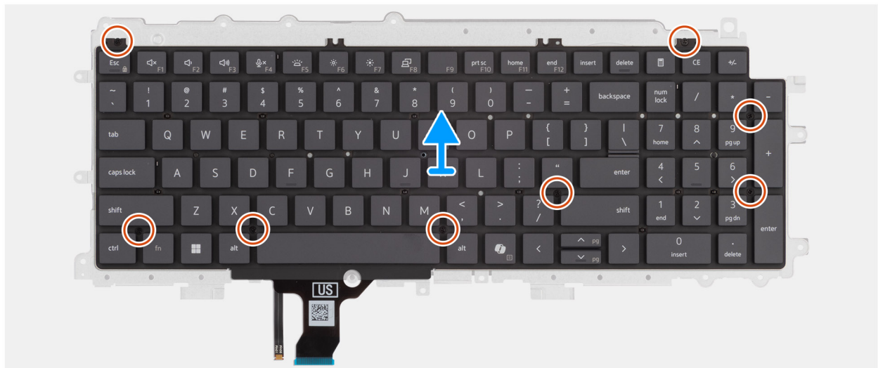
Figure 66. Removing the keyboard support plate
