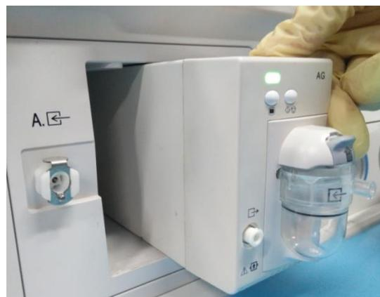
4. Insert one end of the exhaust tube into the exhaust outlet on the module, and rotate it clockwise to tighten it.
