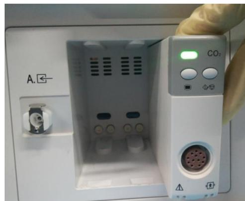
3. According to the triangular mark of the connector, insert one end of the connector into the sample port.
