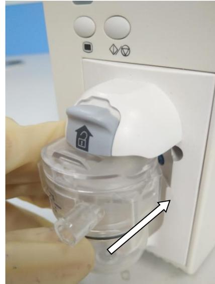
2. Install the module into the module slot.
