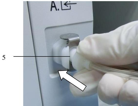
6. Insert the sampling line into the sampling port.
