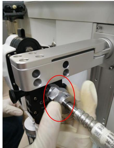
2. Unscrew the four screws between the external vacuum suction system and its support.
