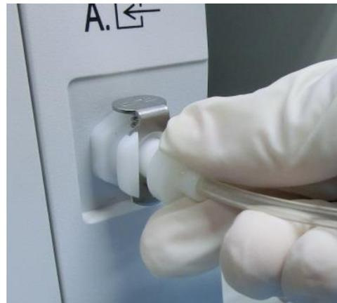
6. Insert one end of the sampling tube into the sampling tube port, then rotate it clockwise to tighten it.
