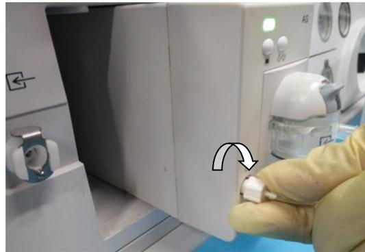
5. Insert the other end of the exhaust tube into the exhaust inlet on the anesthesia machine. A “Click” sound indicates the tube is installed in place.
