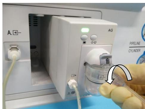
2. Press down the clip at the exhaust outlet of the anesthesia machine to pop out the exhaust tube, and then remove the tube, as shown in the tight figure:
