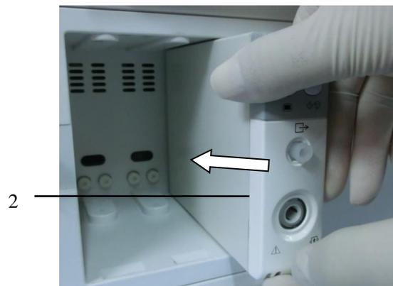
3. The indicator light on the module turns on, indicating the module is installed properly.
