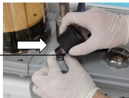
2. When the CPC connector latch is released, pull out the airway gauge.
