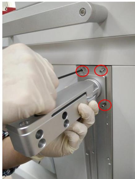
3. Fix external vacuum suction by tightening the four screws on the bracket.
