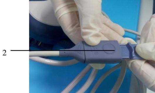
3. Plug the BISx device cable connector into the BIS module connector, as shown in the figure:
